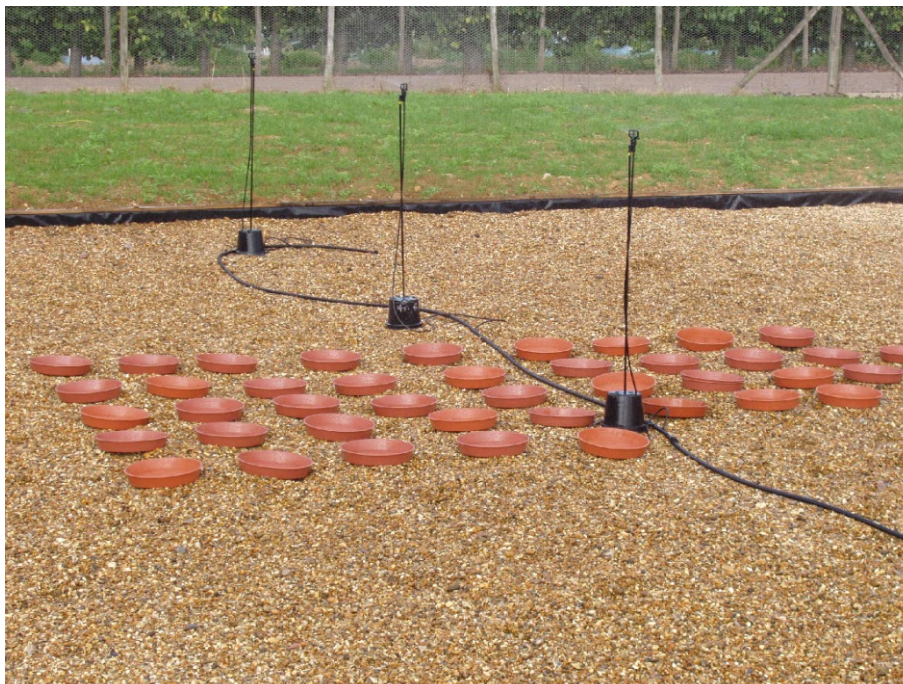
Figure 15: The procedure used to evaluate irrigation sprinkler distribution using the large gravel bed (10 x 30m) at the East Malling Water Centre, 'Catch pots' quantitatively determine the amount of irrigation received and their distribution is used to calculate efficiency and uniformity of application
