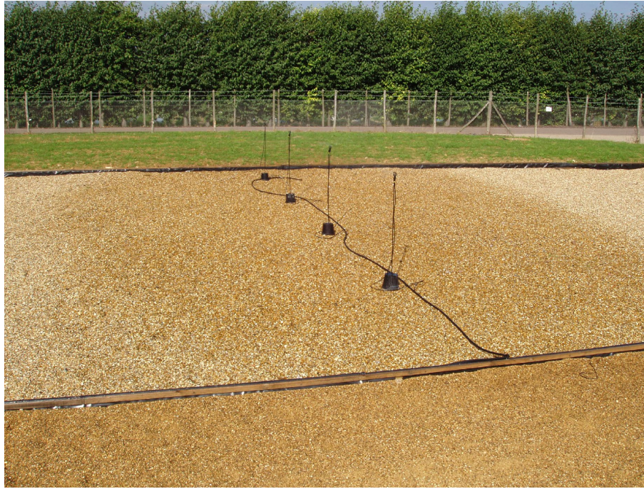
Figure 14: The use of the large gravel bed (10 x 30m) to evaluate irrigation equipments at the East Malling Water Centre, here with overhead sprinklers
